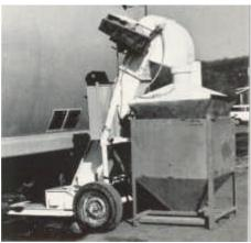
Model 1210 Portable Railcar Unloader unloading talc from railcar to be used in manufacture of roofing shingles.
